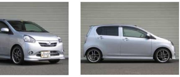
\*For vehicles manufactured on or after January 1st, 2006, if the lower edge of the fog light is less than 250mm from the ground when lowered, it may not comply with Japan's vehicle safety regulations. Please adjust the ride height to secure the minimum 250mm clearance. For details on inspection standards, please contact the nearest National Agency of Vehicle Inspection.
